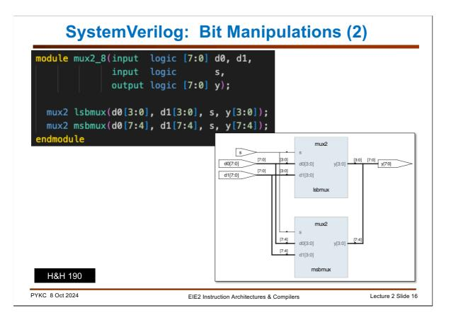
This is an example of slicing and merging different bits of signals d0 and d1 to form an 8-bit output y.
