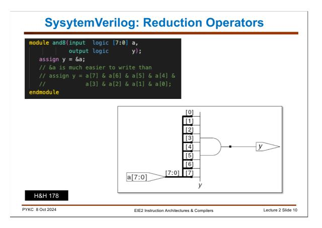
The '&' operator can also be used with a single operand as shown here. This is called a "**reduction**" operator. It reduces multiple bits of a[7:0] to a single bit y. It basically ANDs all bits of a[7:0] together as shown in the slide.
