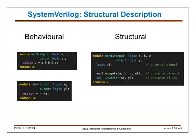
Combinational circuit is easiest to specify using behavioural specification with Boolean operators. You can also choose to provide structural description with interconnected gates as shown on the right.
