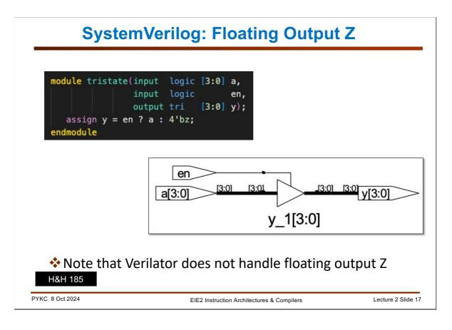
We normally use "**logic**" to specify a signal to be a signal which has values of 0 or 1. However, there is a signal type **tri** which can take on three values: 0, 1, or z, where z is high impedance. This allows SystemVerilog to **describe tri-state outputs**.
