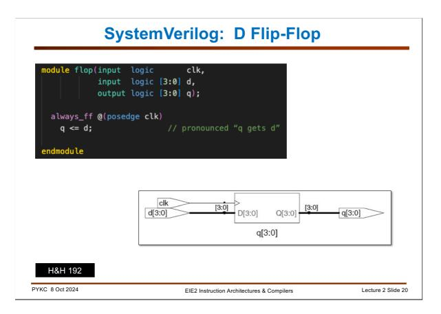
SystemVerilog has a specific syntax for D flip-flops.
