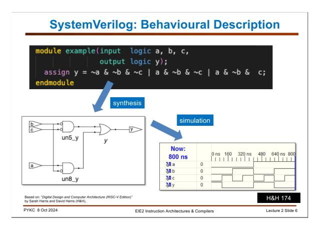
Here is a simple example of a combinational circuit consisting of many Boolean operations described in SV as a Boolean equation. We use the "**assign**" keyword to specify combinational circuit. We then use ~, & and | for NOT, AND and OR Boolean operations respectively.
