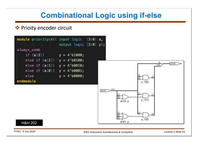
Here is another example called **priority encoder**. **always\_comb** statement uses **if-els**e constructs. The output y[3:0] reports the position of the first '1' in the input from MSB to LSB. So if a[3] is '1', then y[3] is '1' etc.
