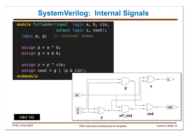
For most modules, there are internal signals which are neither inputs nor outputs. The module here is a single bit full adder. There are two internal signals p, g.
